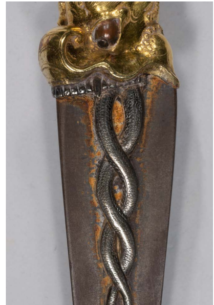
Fig. 3. Acc. no. 52.311 : Rust on the iron blade caused by residual silver-polishing products.
